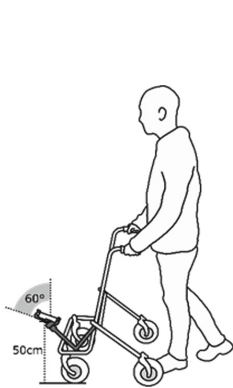
Fig. 1. The data collection apparatus, including the smartphone positioning
